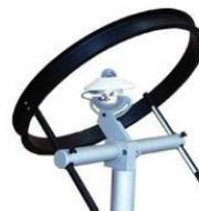
In combination with a pyranometer, the shadow ring allows measuring diffuse radiation. A second pyranometer measures global radiation. Direct radiation = global radiation – diffuse radiation (For more precise measurements, tracking systems with pyrheliometers are used.)
